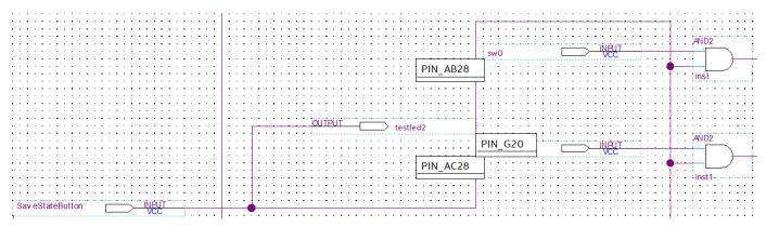
The **SaveStatebutton** which is set to **KEY2** on the FPGA works in tandem with the switches to ensure that tone data is not saved into one of the **4bitregisters** without the user enabling it. To do this the **SaveStateButton** is wired into twelve and gates along with each switch. Gating the output, and enabling/disabling the registers.
