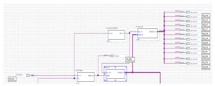
Once the system's native clock frequency is slowed to 180bpm the output signal goes into the **Sequencer**. The **sequencer** much similarly to **FourBitButtonIncrementCounter** increments 12 times and resets on each rising edge of the newly generated 3hz signal. The **sequencer** outputs a 4bit bus into a module **LED\_Sequence** controlling turning on the LED's and into a select input of the **12-1MUX** below.
