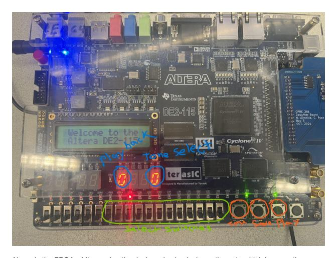
Above is the FPGA while running the device, play back shows the note which is currently saves at each beat, **tone** select shows the note you want to save onto each beat, and the **tone** button cycles through 0 - 12 corresponding to the tone, holding down **save**, saves a tone to the **switches** you have engaged, and **play** starts and stops the sequencer.
